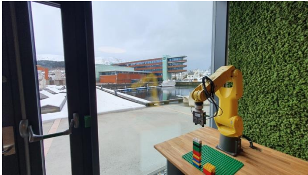
A robot in the maker lab demonstrating the assembly of a unit of LEGO pieces.
